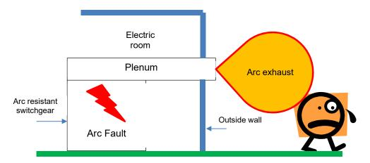
Figure 9. Inadequate arrangement of external arc venting system
