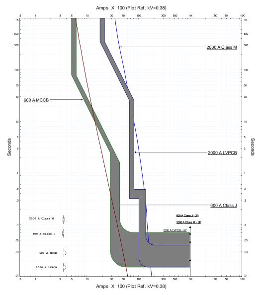
Figure 1. Time–current characteristics of four low voltage elements for the assessment of device limited ratings of arc-resistance equipment
