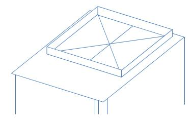
Figure 5. Flap plates on an arc-resistant device, typically closed
