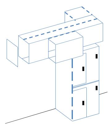
Figure 8. Common arc-resistant medium voltage container with plenum
